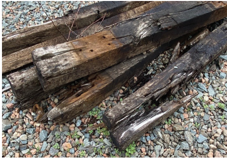
Creosote treated wood
